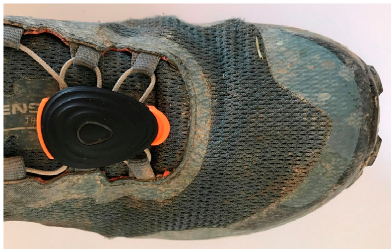
Figure 3. The Stryd sensor fixed on the right shoe of one of the participants.
