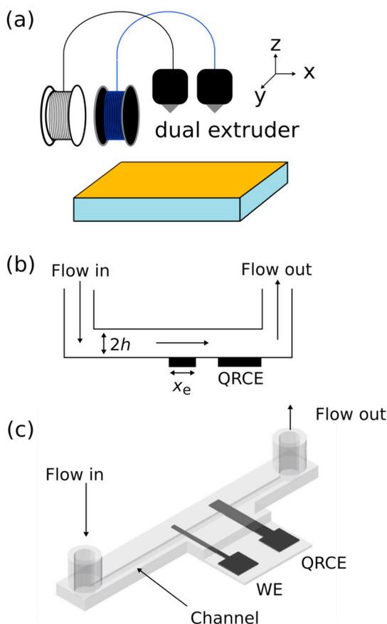
**Fig. 1.** Schematic of the experimental setup and devices. (a) schematic of dual extrusion 3D printing setup with two materials; (b) schematic representation of the channel flow geometry and the positions of the two electrodes. This schematic is not to scale; (c) CAD drawing of a channel flow cell with a  $1.5 \text{ mm} \times 1.0 \text{ mm}$  channel and two band electrodes.
