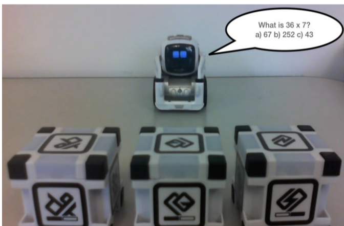
Figure 1b. Physical Embodiment. Here TIPPAE interacts with the student through a robot. The student can respond to TIPPAE's questions by selecting one of the block's placed in front of the robot. If the answer is correct, TIPPAE responds by exuberantly moving around.
