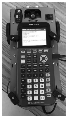
Figure 16. Rover a car that attaches to a programmed graphing calculator
