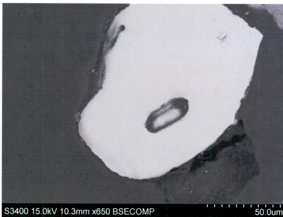
Figure 7A. Homogeneous Texture. There are no visible exsolution bodies or noteworthy features on, or within, the grains. This example is an ilmenite grain. The oval feature is likely a scar from plucking out another mineral grain (WAW2 near Recovery Ice Stream).
