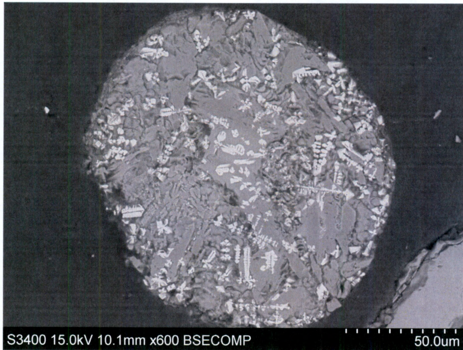
Figure 7G. Extrusive igneous texture. This term describes Fe-oxides within basalt lithic fragments. The Fe-oxide grains (bright white) are euhedral or have skeletal crystal forms. This example is a basalt lithic clast containing multiple skeletal magnetite crystals (YAR4A from Foundation Ice Stream).
