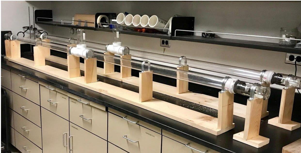
**Figure 1.** Apparatus A and B. Mosquitoes were introduced to the tube in the top, center, jar. A light was placed at one end of each tube, on the outside of blackout material. Holes were cut into the material to let in a limited amount of light. Collection jars at either end of each tube held mosquitoes. Exiting the jar was inhibited by the funnel shape of the entrance.
