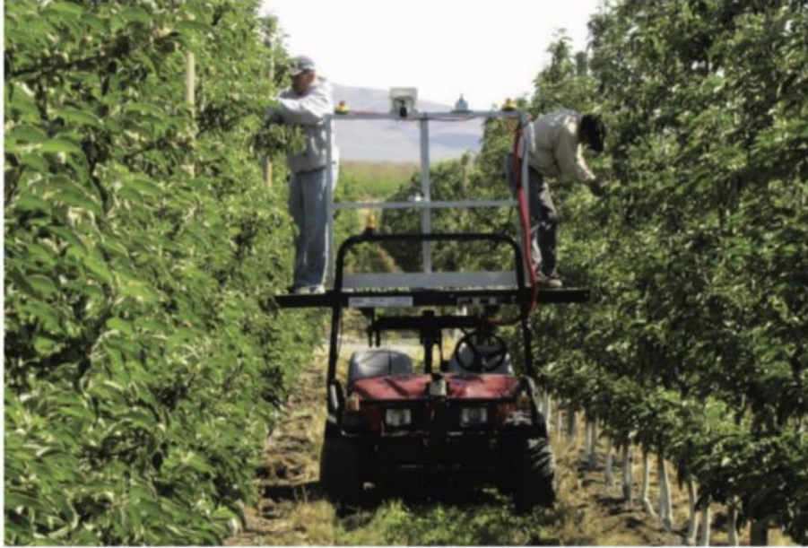
Figure 7: Workers using a robot vehicle that acts as a platform for tree fruit farming [26].
