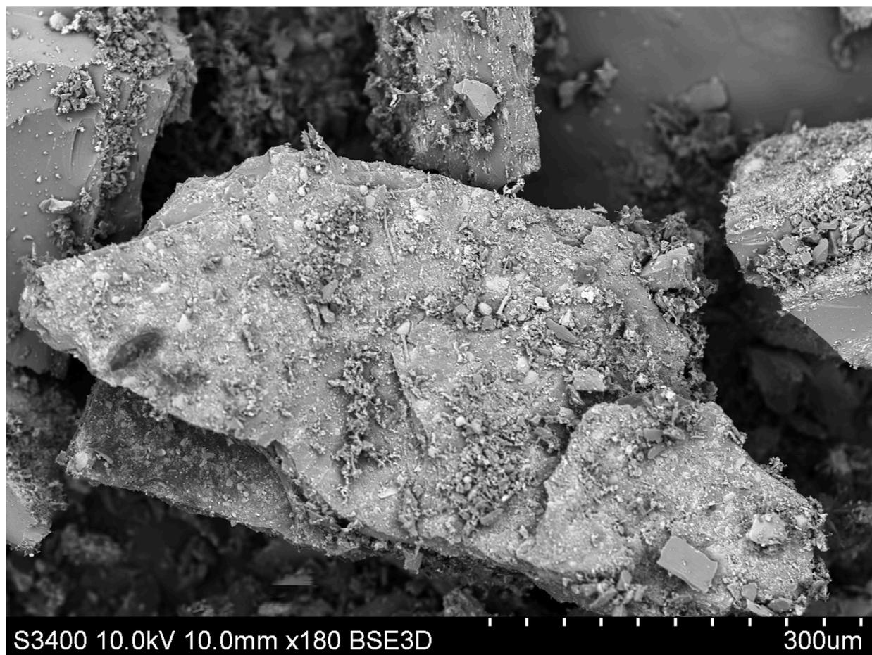
**Figure 3-6.** Scanning electron micrograph of fragments of a single wet-sieved ( $> 2$  mm) and sonicated LSP 43 coal particle. Note surface encrustations. Scale bar is 300  $\mu\text{m}$ .
