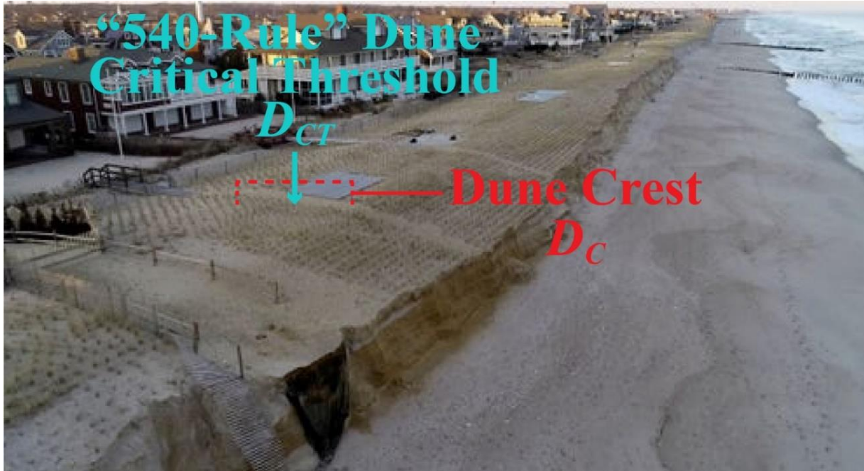
Figure 3.8 - Example of a “540-Rule” dune’s critical threshold location following a dune scarping event (Bay Head, NJ).
