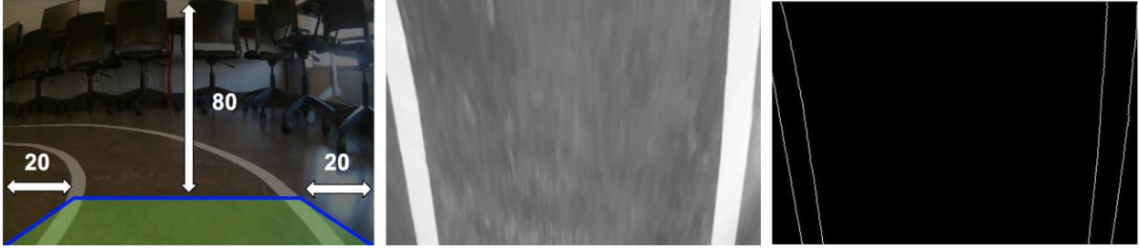
Figure 14 1/10-scale vehicle image transformation perspective.
