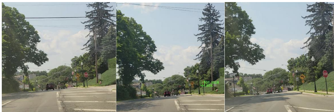
Figure 26 Stop sign recognition approaching a tilted sign facing a different direction at far distance. The algorithm performed the worst under these conditions.
