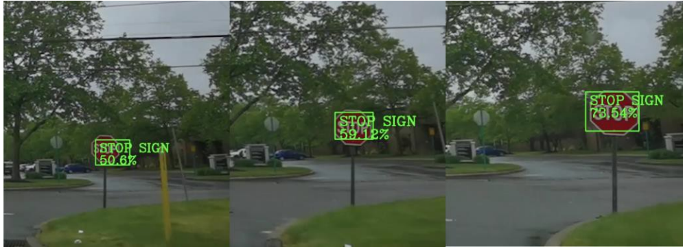
Figure 24 Stop sign recognition algorithm performance based on front-facing stop sign at closer distance. The algorithm performed the best under these conditions.
