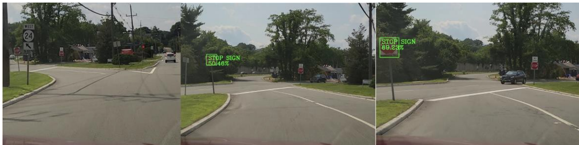
Figure 25 Stop sign recognition approaching stop sign on a curve road.
