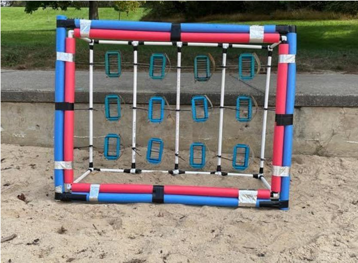
Figure 2: Photo of Floating Island Rig System with Periphyton Samplers
