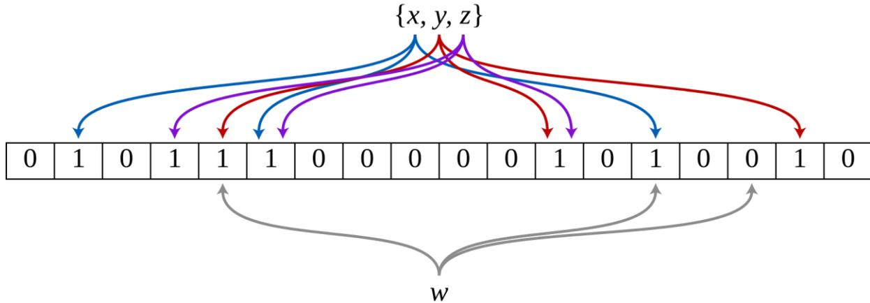
**Figure 2: Example of a Bloom filter**
