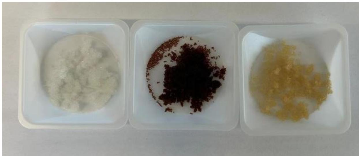
**Figure 5-4** Visualization of fresh IRA67 (left), IRA67 with no regeneration after six cyclic adsorption-regeneration tests (middle), and ARP regenerated IRA67 after six cyclic adsorption-regeneration tests (right)
