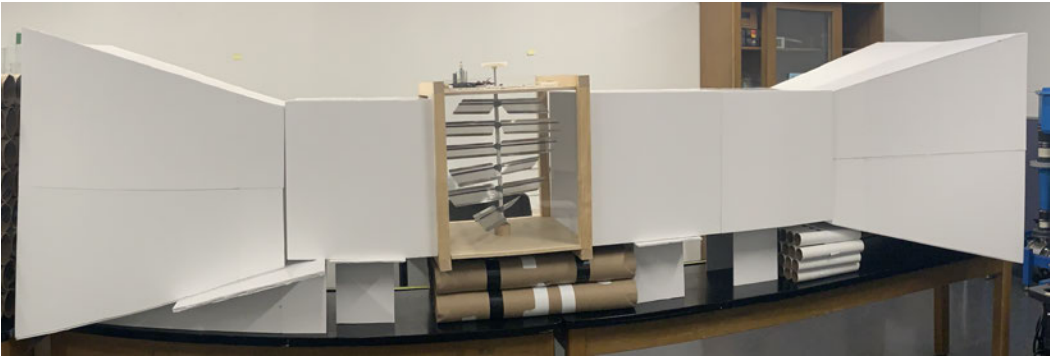
(b) Constructed wind tunnel
