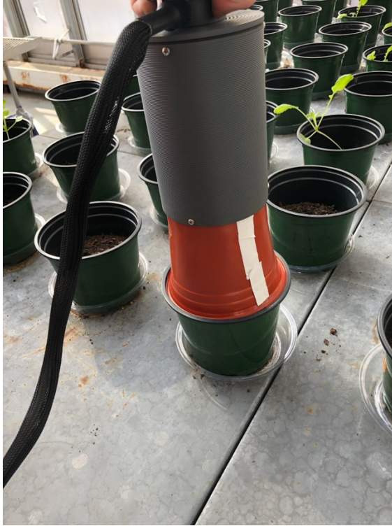
Figure 1: Once seedlings reached a height such that the EGM-5 gas analyzer could not be applied without damaging plant tissue, an additional vertical chamber was fitted to the chamber as shown.
